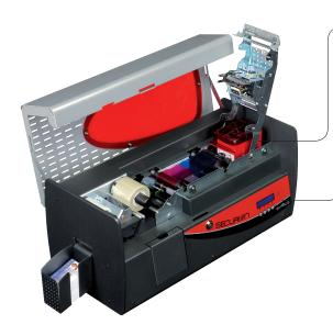
Blank card storage in a removable feeder with a capacity of 100 cards
