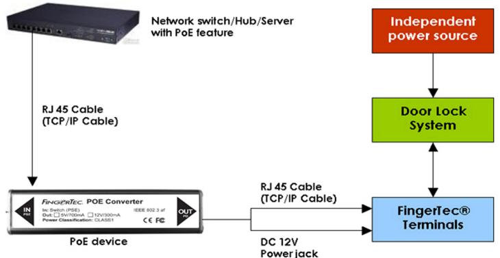
The PoE device can only use to power on and to communicate with the FingerTec® terminals. Its power is not strong enough to support door lock system. Therefore you must have an independent power source to power on the door lock system. The FingerTec® terminal will interact with the door lock system to control accessibilities of users. You can replace the "independent power source" with AdapTec® AC, as it can support a backup battery.
