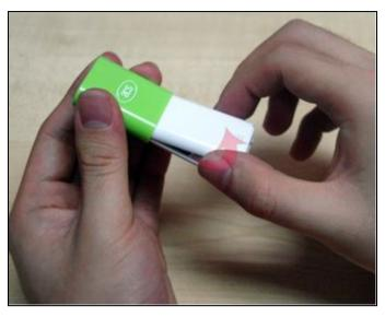
Remove the cover to reveal the SIM-sized card and Micro SD slot.
