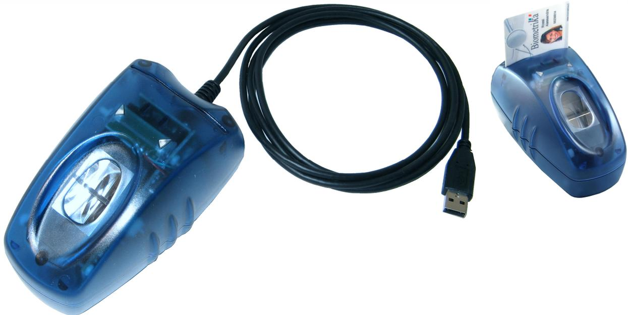
Fx2100-basic is a FTIR optical fingerprint scanner, which, thanks to its powerful CPU is capable of performing in hardware several useful tasks, thus improving security, efficiency and usability. The accurate optical design allows high quality images to be captured and a large finger area to be sensed.
